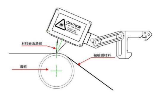
This is the way the CCD camera and the roll are in a certain angle, istance roller about 30mm, This case is mainly applicable to the tracking of the laser film and some weak contrast conditions.
