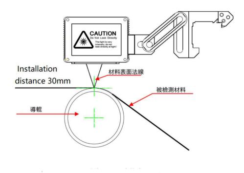
This is the way the CCD camera is perpendicular to the roll, Distance roller about 30mm, This case is mainly suitable for tracking transparent film. High reflective material. The situation of high contrast materials.
